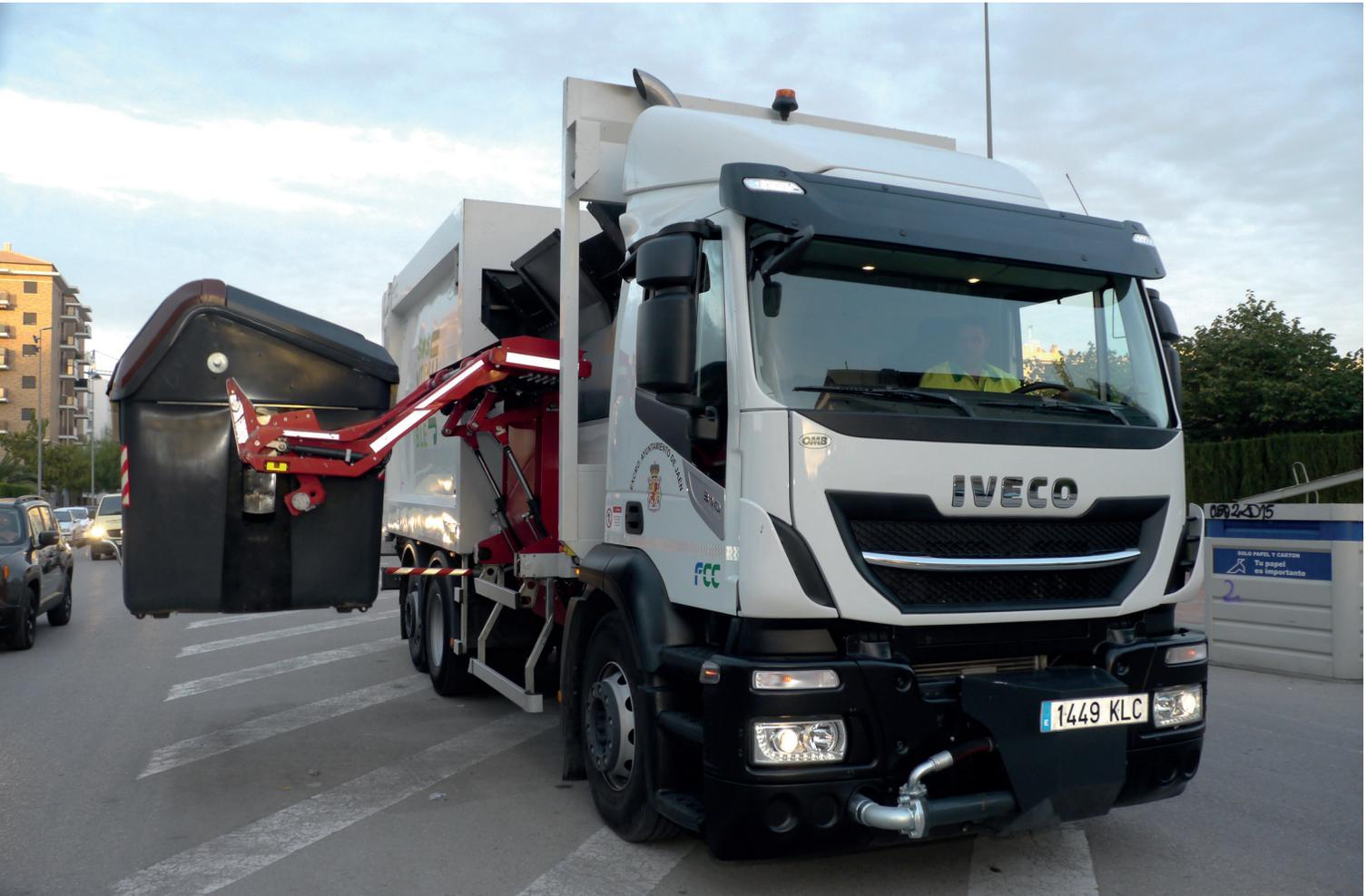
To improve the service, FCC will be introducing a side-loading waste collection system to replace a large part of the current rear-loading system.
